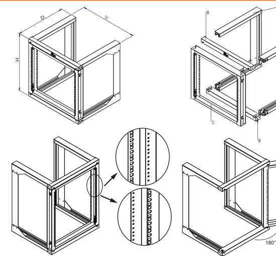
Pre-tapped 12-24 threaded holes on one side and square rack holes on the other. According to the installation requirements choose threaded or square at front.
